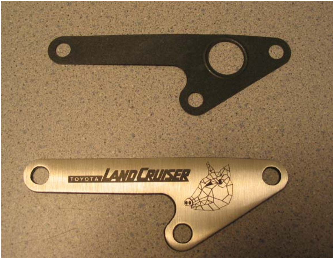
Intake manifold EGR gasket and stainless steel block-off plate. Plate can be easily cut to match the gasket by a local sheet metal shop. Obviously the laser etching isn't necessary, but it does add a nice finishing touch.
