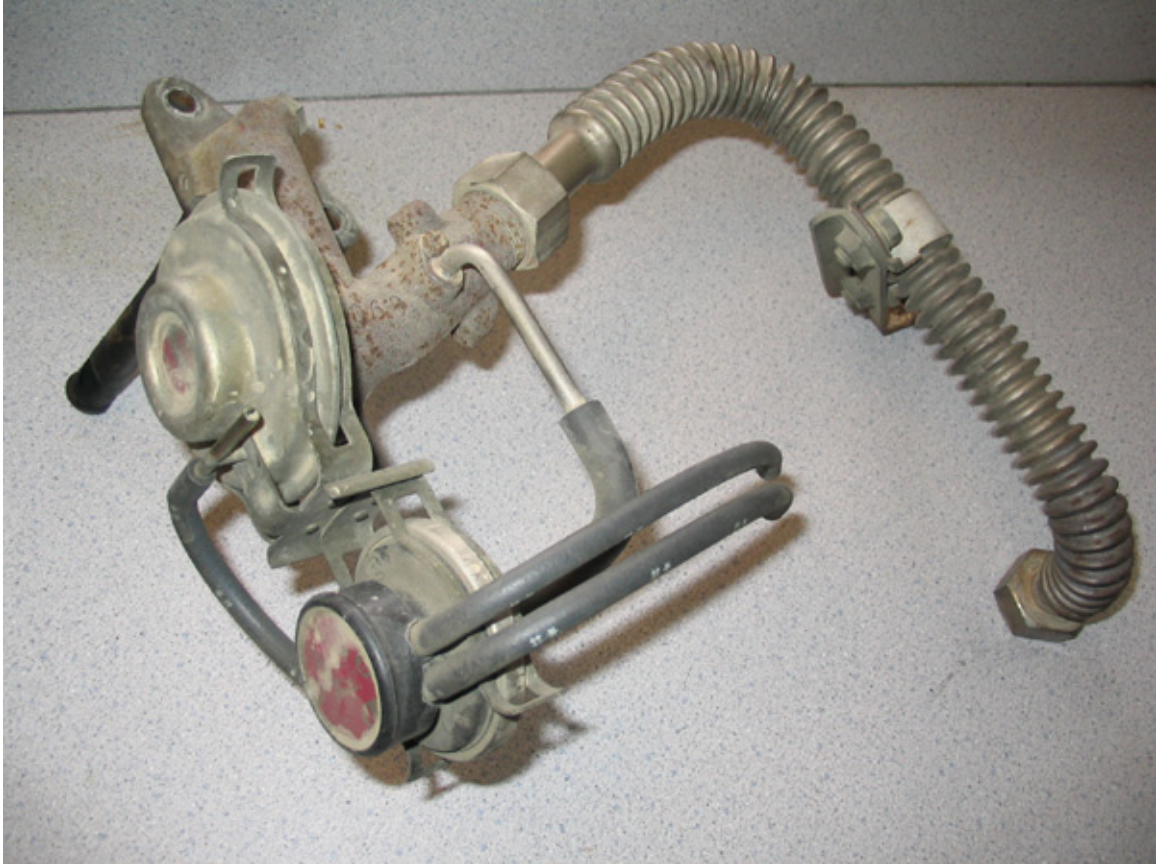
The entire EGR assembly removed from my truck. That black tube that extended into my intake manifold was very thickly caked with nastiness.
