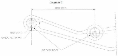
5. Install the second bush by positioning the bush pin centre at the same centre spacing previously taken from the original bush centres in 2. above.
