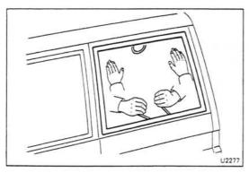
(c) From the inside, pull on one cord at an angle so it pulls the lip over the flange. From the outside, press the glass along the weatherstrip until the glass is installed.
