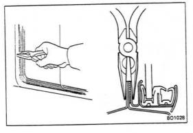
(e) To compress the butyl tape, squeeze the sash and body edge portion together with pliers.
