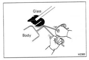
(c) From the inside, pull on one cord at an angle so it pulls the lip over the flange. From the outside, press the glass along the weatherstrip until the glass is installed.
