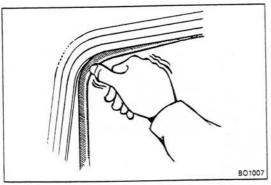
(f) Install the sash clip on the body and outer sash edges.
