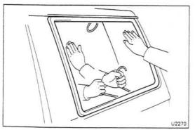
(d) From the inside, pull on one cord at an angle so it pulls the lip over the flange. From the outside, press the glass along the weatherstrip until the window is installed.
