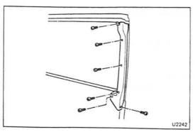
INSTALL BACK DOOR CONTROL LINK COVER Install the link cover with six screws.
