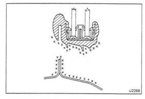
(b) Apply soapy water to the contact surface of the weatherstrip lip and to the body flange.
