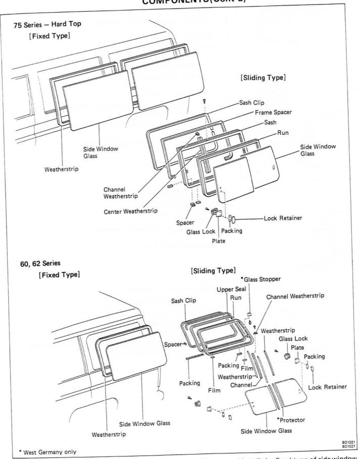
NOTE: Remove and install the fixed type of side window on the back door glass with the same procedure. (See page BO-66)
