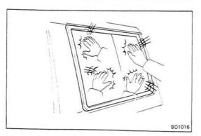
(e) Tap on the outside of the glass until it is securely in place.
