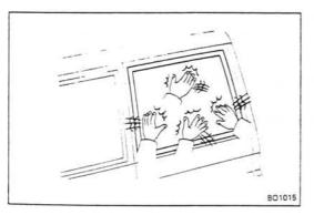
(d) Tap on the outside of the glass until it is securely in place.
