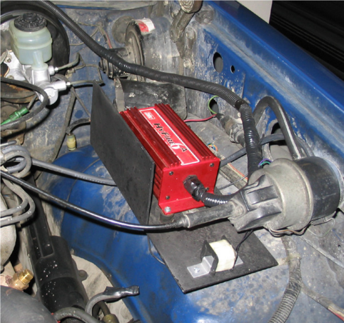
Fender space freed up (and used) after removal of the solenoid assembly and VSV. I saved the flat bracket and mounted my ignition mount/heat shield to that. The cylindrical part you see just forward of the ignition is the actuator for my cruise control.
