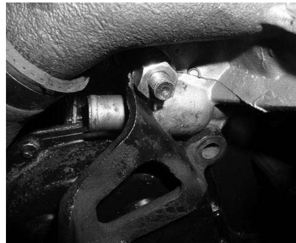
The idler pulley for the large belt had to be ground a little to clear the water pump outlet.
