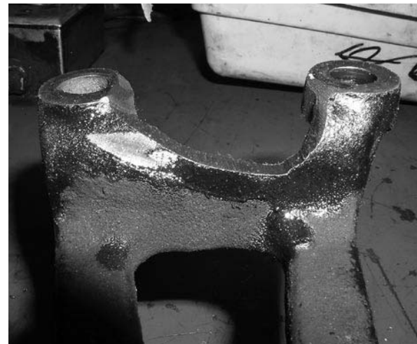
A clear view of how much material was removed from the idler pulley bracket.
