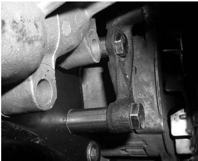
The upper mount for the alternator previously bolted up to the water pump but is now mounted to the block using spacers made from 3/8" pipe.
