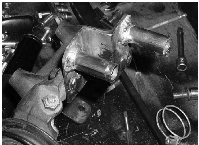
A/C to power steering adapter bracket bolted to the A/C mount.
