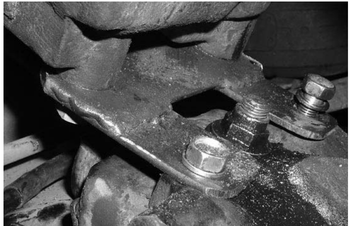
To clear the water pump main outlet I had to move the A/C pump out 2-1/4". This is the mount that I made from 1-1/2" x 1/8" steel, drilled to match the A/C pump mount.
