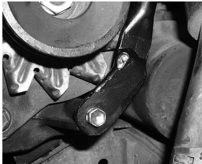
I extended the smog pump support brace using 1" x 1/8" stock doubled up and kept it as low as I could so that I could use the original hoses.
