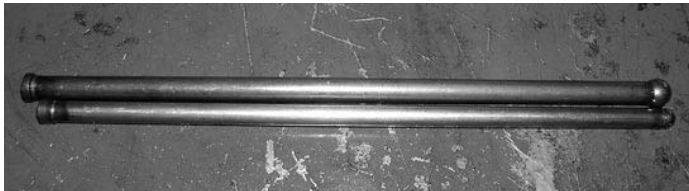
I used pushrods from a 2F. The top one is from a 1975 2F and the bottom one is from the 3F-E. I used new ones from Clevite (PN 21-3270) that are intended for the 2F.
